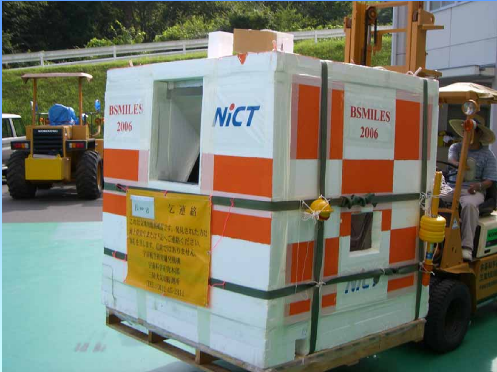
Thermal insulation : 100-mm thick Styrofoam
