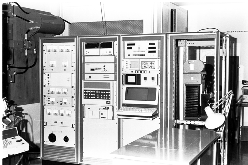
Fig. 6. The Auroral Observatory ionosonde (Larsen and Berger, 2000).
