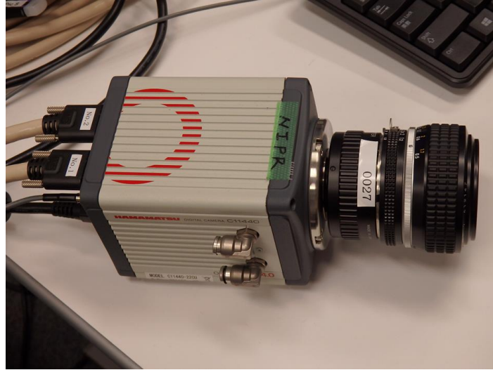
Figure 2.1: sCMOS camera (ORCA-Flash 4.0 V2, Hamamatsu Photonics) equipped with a NIKKOR 50 mm/F1.2 lens.
