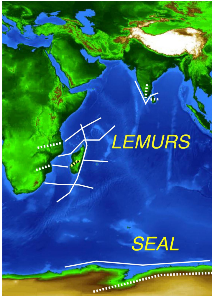
Figure 4: Present-day continental configuration, with example of a possible program for deep seismic surveys at sea (solid) and on land(dashed). Actual survey routes will require careful scouting and planning, and will exploit both active and passive methodologies and opportunities for integrated onshore-offshore acquisition. These routes, which are only loosely related to those in Figure 3, are primarily intended to convey the scale of such a program.
