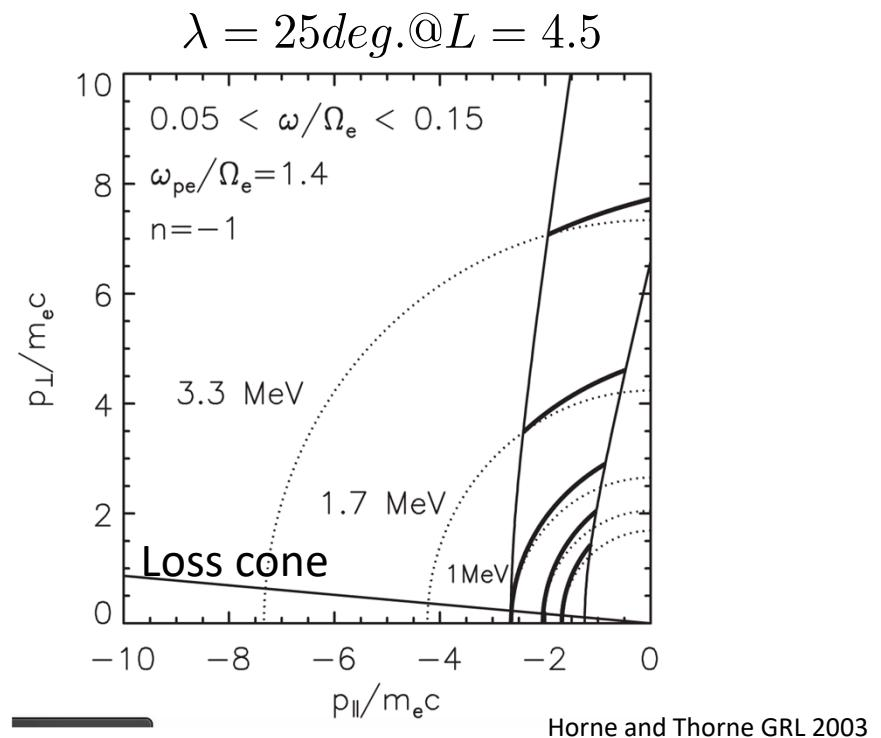
Higher energy electrons at loss cone angle can resonate with whistlers at higher latitudes.
